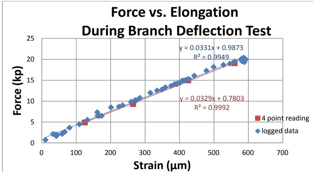
**Figure 5. High correlation between deflection, fiber strain, and force indicating that tests were made in the range of elasticity of the branches.**
