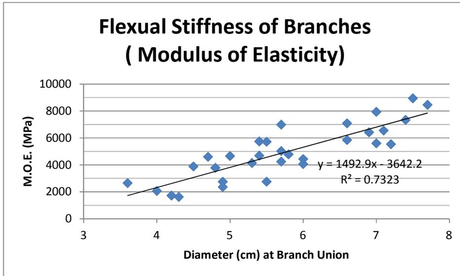
Figure 14. Correlation between branch diameter and elasticity.
