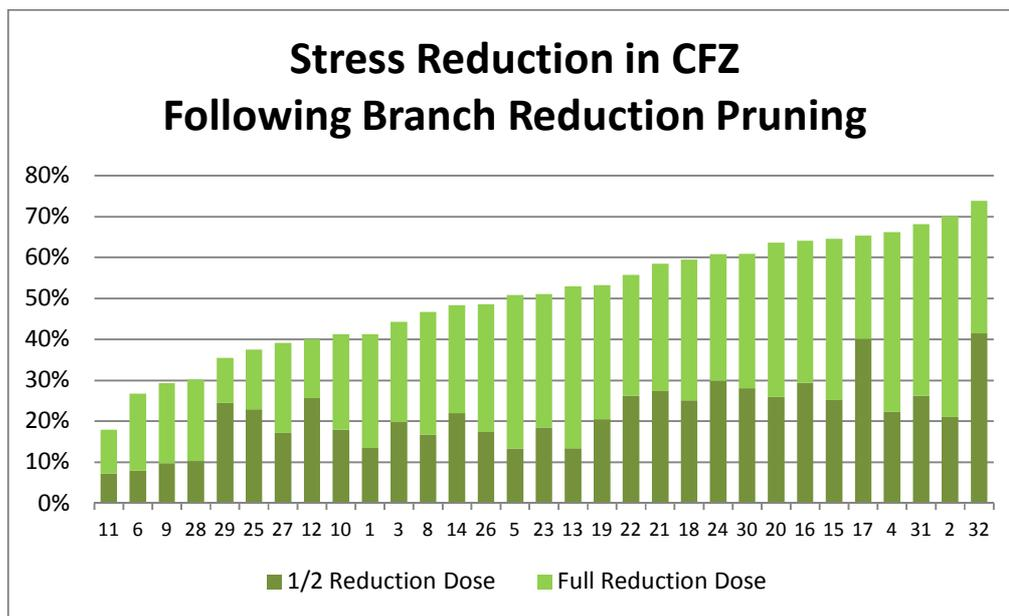
**Figure 10. Reduction in bending moment following branch reduction pruning in the region where the branch is most likely to fail structurally. Numbers on x-axis indicate test number.**
