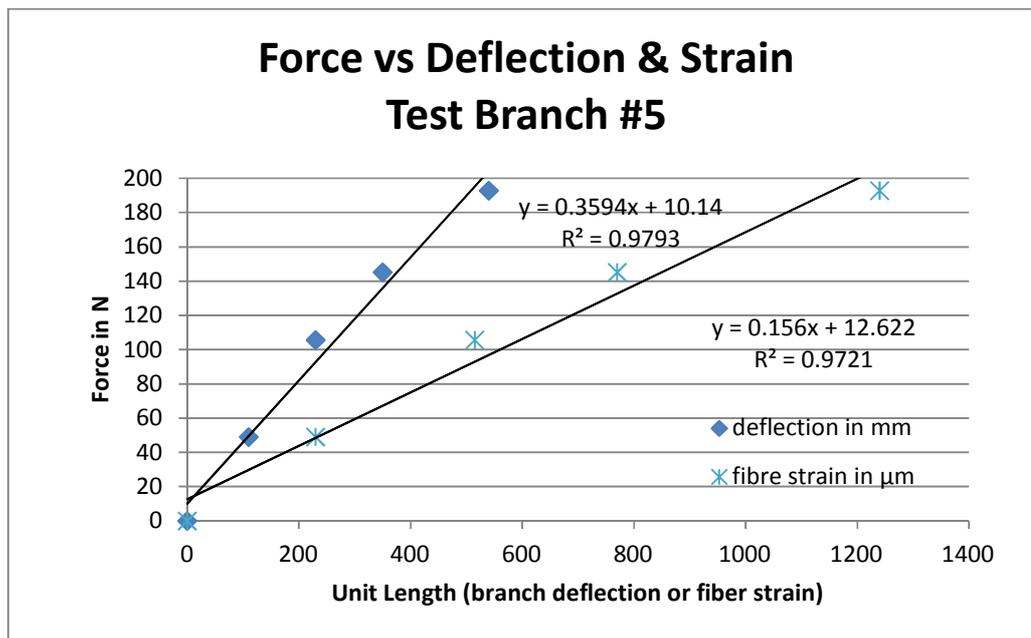
**Figure 6. The relationship between force and both deflection and fiber strain indicate elastic limit may have been reached.**
