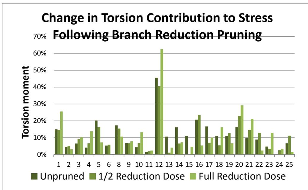
**Figure 15. Relationship between reduction pruning and torsion moment as a percentage of bending moment. Numbers on x-axis indicate test number.**
